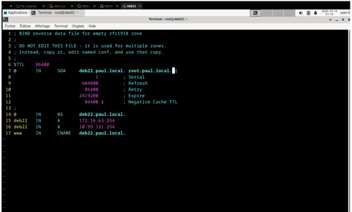
A terminal window showing the configuration of a BIND reverse data file for the paul.local zone. The configuration includes SOA, NS, and A records.
