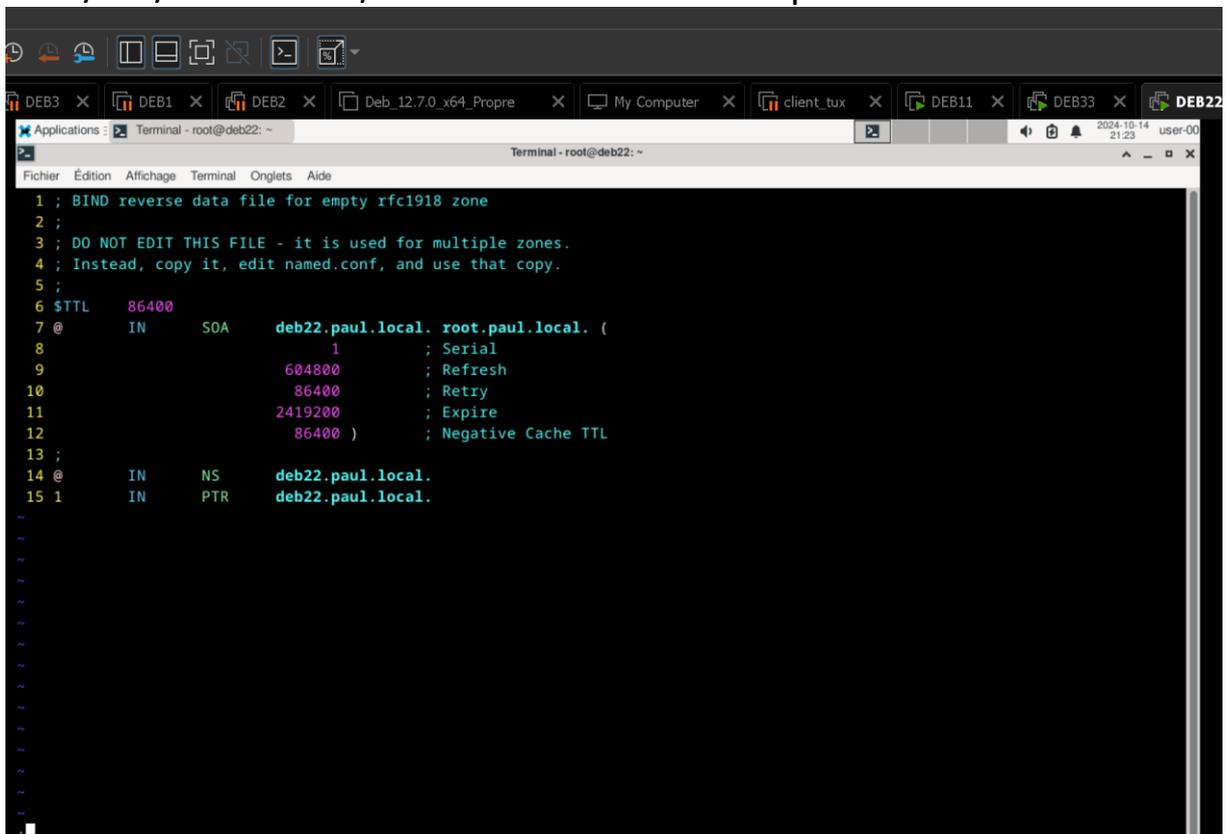
A terminal window showing the configuration of a BIND reverse data file for the 172.16.63.254 zone. The configuration includes SOA, NS, and PTR records.
